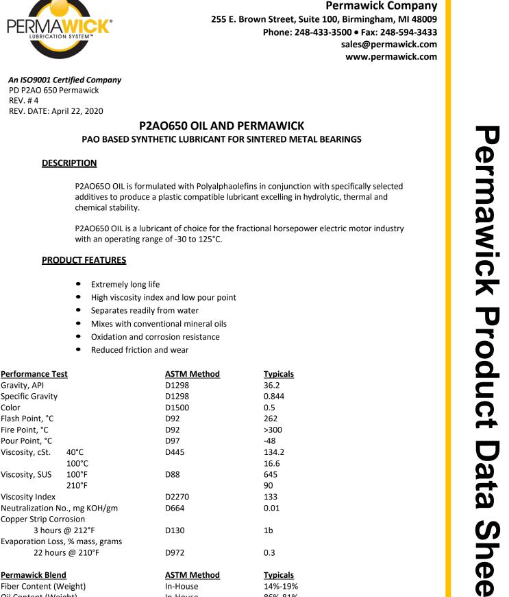
Color Flash Point, °C Fire Point, °C Pour Point, °C Viscosity, cSt. 100°F D88 645 Viscosity, SUS 210°F 90 Viscosity Index D2270 133 Neutralization No., mg KOH/gm D664 0.01 Copper Strip Corrosion 3 hours @ 212°F D130 1b Evaporation Loss, % mass, grams 22 hours @ 210°F 0.3 D972 **Permawick Blend ASTM Method Typicals** Fiber Content (Weight) 14%-19% In-House Oil Content (Weight) In-House 86%-81% **Moisture Content** D95 <1.6%
